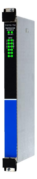
The 7070TM module processes six temperature sensor inputs, including Resistance Temperature Detector (RTD), Thermocouple (TC), and Thermistors. Flexibility is inherent in the design with the ability to configure any input channel for any type of supported temperature sensor. By utilizing modern digitizing circuitry, the 7070TM offers laboratory level accuracy in an industrial package.
