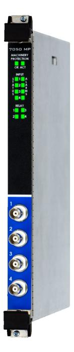
The 7050MP Machinery Protection module combines the features found in a traditional protection cards with the advanced analysis of portable systems.
